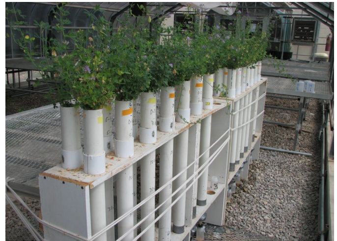
Greenhouse soil column study evaluated cooling tower reject water irrigation effects on alfalfa performance, soil salinity, and leachate chemistry.
