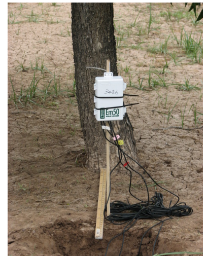
Example of a soil moisture sensor installed in the field
