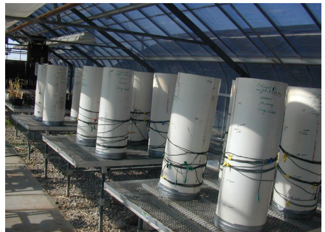
Bench-scale soil column tests
