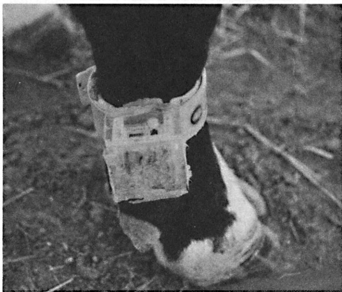
Fig. 1. Pedometer enclosed in a plexiglas case that is attached to a cow's foreleg.
